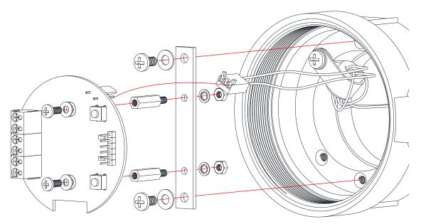
The DCS head is provided with a cable gland for cable diameters between 6 and 8mm. For smaller diameters cable, replaced with a suitable sized M20x1.5 gland.
