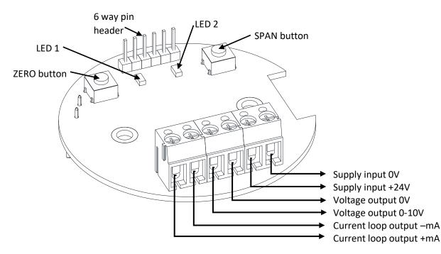
The sensor outputs the float level as a varying voltage or varying current. Connection can be made to voltage, current or both voltage and current outputs.
