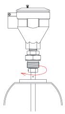
A DCS with a short sensing length can be mounted horizontally to give a binary level indication. When mounting horizontally ensure the breather holes aligns vertically to allow the liquid to drain from both the top and bottom of the stem.
