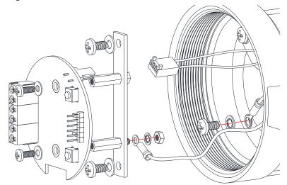
If required, both the cable screen and chassis may be connected to the metal pillars as described above.
