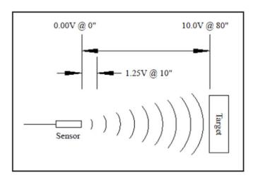
The RPS-409A-IS3 is an intrinsically safe analog ultrasonic sensor available in a variety of ranges. The RPS-409A-IS3 sensors can be used in hazardous gas or dust environments classified as Class I, II, or III when used with approved intrinsic safety barrier(s). See the RPS-409A-IS3 User Manual and Control Drawing No. 14122606 for further information on installation in hazardous locations.
