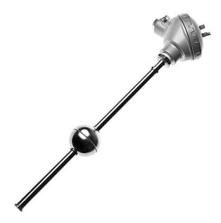
The LVCS is a liquid level sensor featuring a float that can move vertically along a stem. Sensors in the stem detect small step-changes in level and, particularly over longer lengths, the output approximates to a continuous analogue signal.
