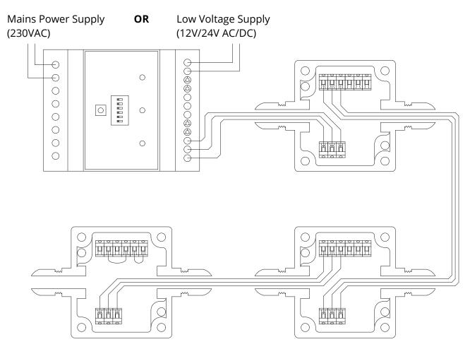
Please note that although a break in the wires connecting the sensors will be detected automatically, in the unlikely event of a sensor failure, there will be no indication of a fault. All Leak Sensors should therefore be tested periodically to confirm that they are functioning correctly by placing the probes in the fluid they are required to detect.
