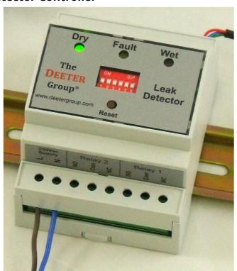
The Leak Detector Controller is housed in a UL94-V0 flame retardant case that will fit to standard 35mm DIN rail.
