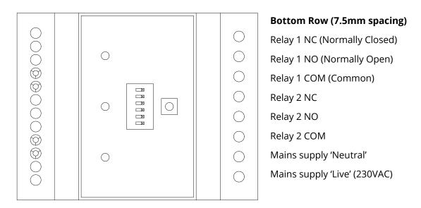
The bottom row (7.5mm spacing) may be used for connecting mains-supply voltages (220V-240V) **or** low voltages if the Controller is not powered by mains. (Mixing mains and low voltages on the bottom row of terminals is not recommended for electrical safety reasons).
