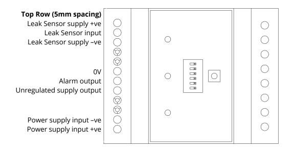
The top row (5mm spacing) has terminals grouped in twos and threes according to function and are used for low-voltage connections only (less than 50V).
