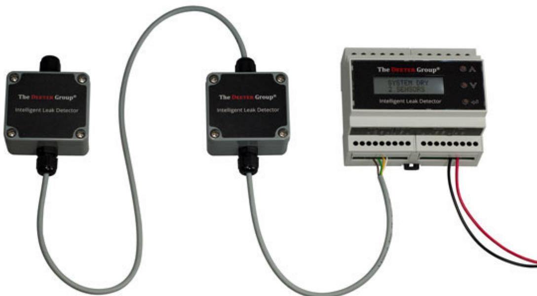
The Deeter intelligent Leak Detector system comprises a leak detector controller in a DIN-rail mounting enclosure and a set of leak detector sensors in small, floor-mounting ABS enclosures. The controller can identify each sensor and provide information about the location of a leak whenever a leak is detected.
