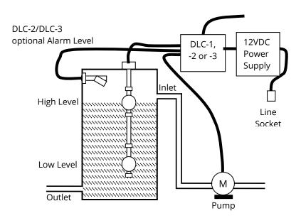
The figure above shows an example where a pump is used to top up a storage tank. Other arrangements can be controlled equally well by the Deeter Dual Level Controller. Please call us to discuss your requirements.
