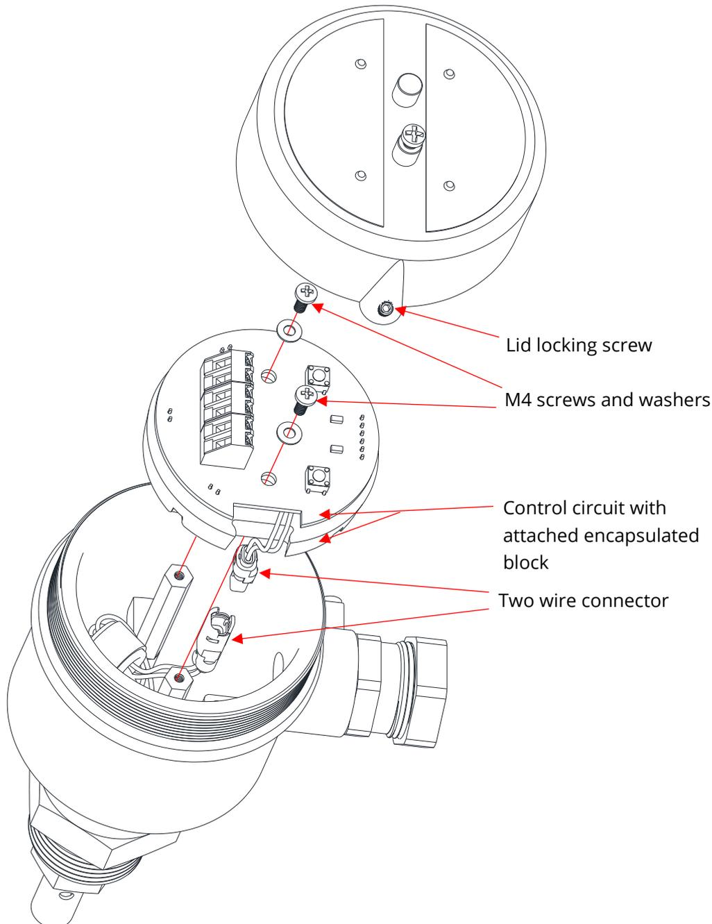
The DCS IS is not normally provided with a cable gland so the installer is free to select an 'Increased safety' cable gland suitable for the temperature and environment around the DCS IS head. The cable entry thread will be either M20x1.5p or 1/2"-14NPT. The product drawing will specify the thread supplied with your model.
