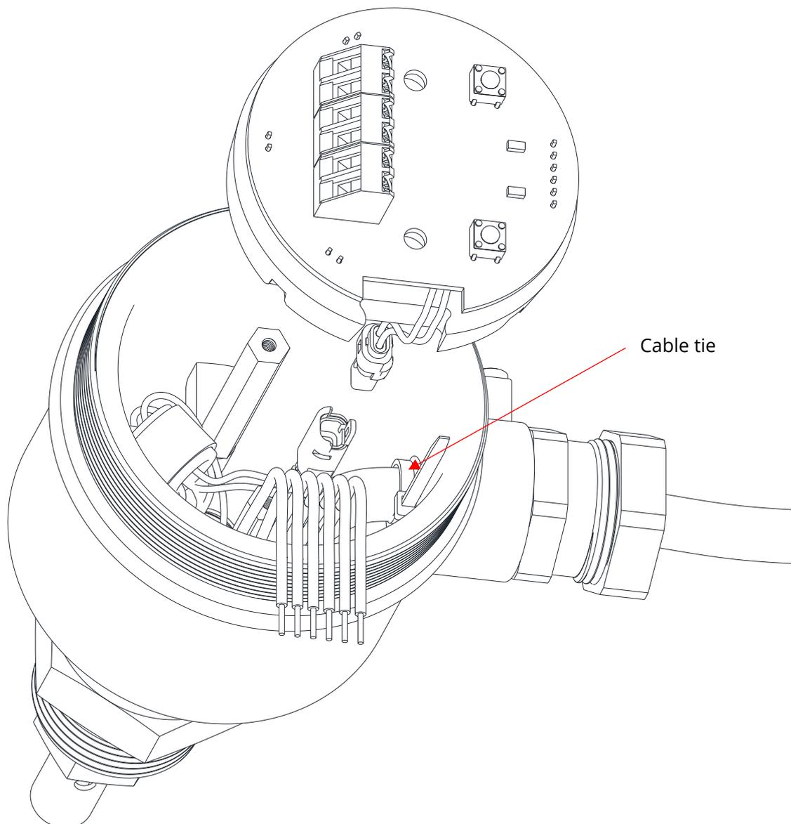
With the circuit board re-fitted back on to the hexagon posts, screw the board down using the M4 screws and washers.
