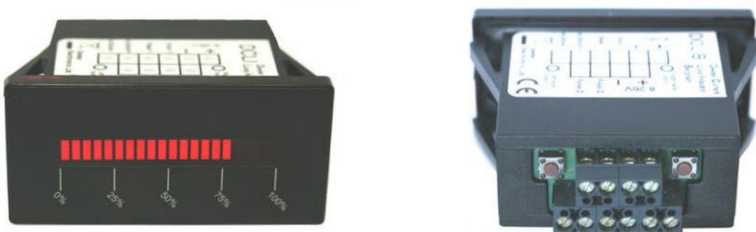
The DCLIB (Deeter Current-Loop Indicator - Bargraph) is an easy-to-mount display module designed to work with any 4-20mA or 0-20mA process sensor. The display consists of a 20-segment bar LED that can indicate the loop current with a 5% resolution\*.
