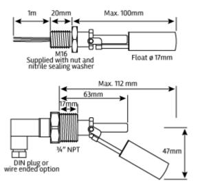
The 80 Series is a small horizontally mounted liquid level sensor designed for high temperature/high pressure operation and sensing chemically aggressive liquids. The design provides a highly cost effective solution where high reliability in a demanding environment is called for. The high temperature version of the 80 series has the added benefit of being able to operate in temperatures exceeding the standard limit of 120°C and can operate in temperatures of up to 200°C.
