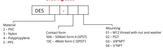
Example: DE53-50A01 describes an M12 nylon sensor having a form A switch rated at 50 watts
